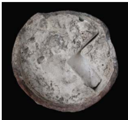
Fig. 2. Top view of crucible 00/0344, filled with corroded and half-reacted glass charge. The trench in the lower right quarter serves to study the internal structure of the filling. The diameter of the crucible is ~15 cm.
